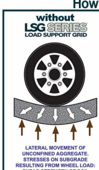
SHEAR STRENGTH OF SOIL **RESULTS IN RUTTING.**
