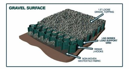
Non-Vegetated / Porous Paving with LSG Series (Load Support Grid)
