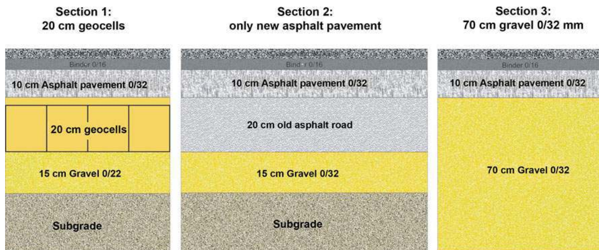
Figure 4: Different reconstruction section, road K-23.
