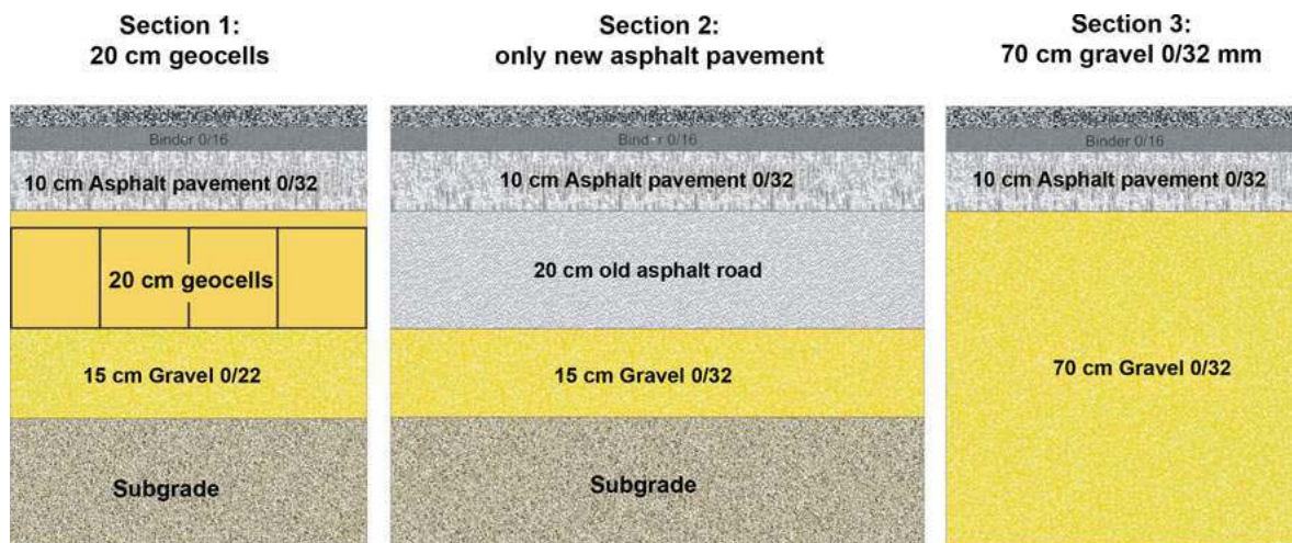
Figure 4: Different reconstruction section, road K-23.
