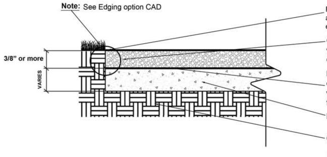
Roller coat of Gravel-Lok<sup>™</sup> liquid (if this is a high traffic area, please add an additional 1-2 roller coats, allowing each one to cure 24 hours in between each application)
