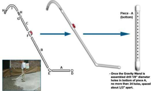
The container that holds the Gravel-Lok liquid needs to be elevated higher than the wand since the flow is achieved by gravity only.
