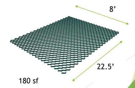
To expand grid to 8' x 22.5' you will need about 16 pcs. of rebar to aid in the process of full expansion. If you are using rebar J hooks in your installation you can use those instead.
