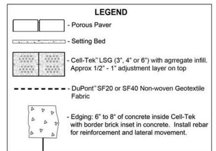
with border brick inset in concrete. Install rebar for reinforcement and lateral movement.
