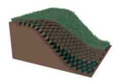
There is a 'correct' and a 'wrong' direction for installing Slope Grid. Slope Grid consists of long strips that are welded together at intervals. The long strips need to be parallel to the hillside.
